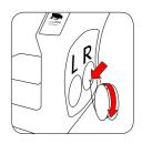
Open the filament hatch by removing the right side panel of the Bolt Pro.
