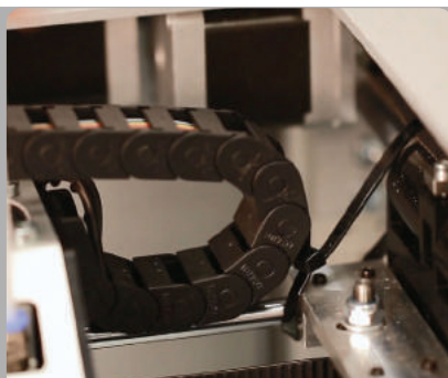
STEP 4: Cut the tie wraps at the front and back of the carriage and in the back of the printer
