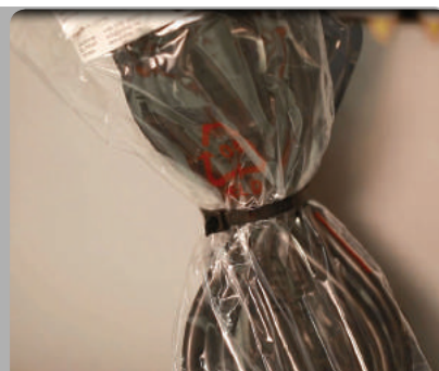
STEP 4: Cut the tie wraps at the front and back of the carriage and in the back of the printer
